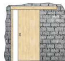
A SINGLE-LEAF DOOR OPENING ALONGSIDE THE WALL
