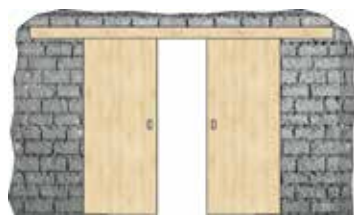
DOUBLE-LEAF DOOR OPENING ALONGSIDE THE WALL
