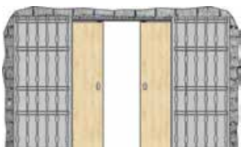
DOUBLE-LEAF DOOR OPENING INTO THE WALL
