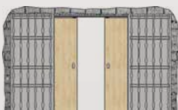
DOUBLE-LEAF DOOR OPENING INTO THE WALL
