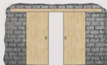
DOUBLE-LEAF DOOR OPENING PARALLEL TO THE WALL
