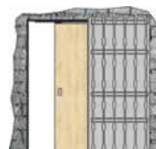
A SINGLE-LEAF DOOR OPENING INTO THE WALL
